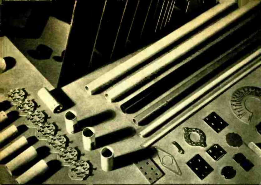
RADIO PARTS OF LAMINATED PLASTIC, WITH POLISHED SHEETS AND TUBES. (Synthane Corp.)
